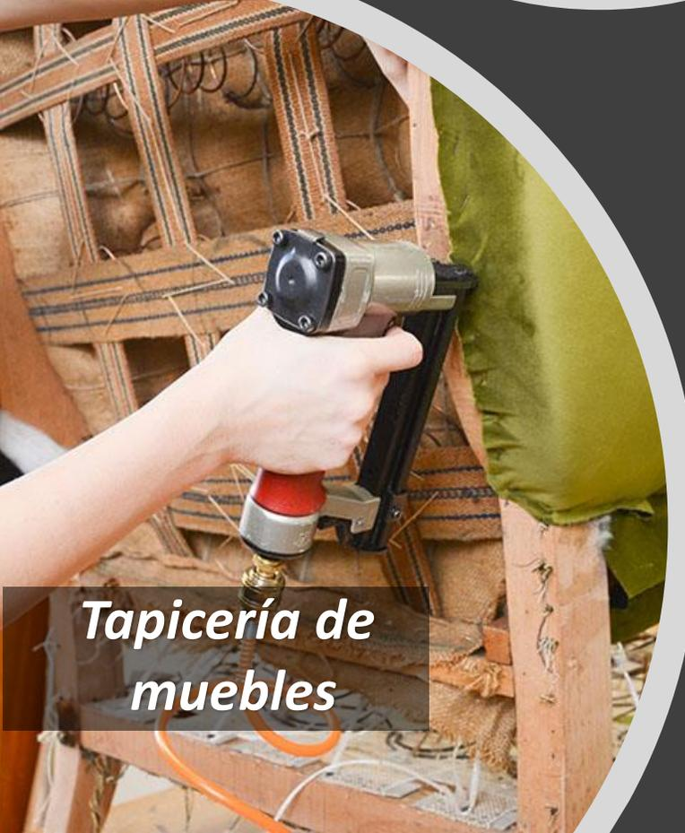
A circular inset image showing a hand using a staple gun to attach green fabric to the wooden frame of a piece of furniture.
